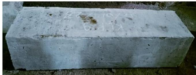
**Gambar 3. 2** Benda uji balok 150mm x 150mm x 600mm
