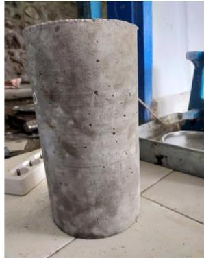
**Gambar 3. 1** Benda uji selinder 300 mm × 150 mm
