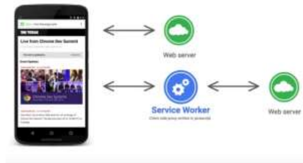
Gambar 2. 4 Cara kerja Service Worker
