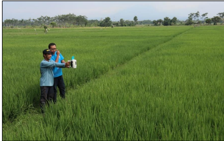
Figure 6. Collecting reference data of spectral reflectance using spectrophotometer.
