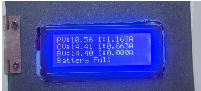
Gambar 5. Pengujian Over Voltage
