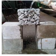
Gambar 1. Beton berpori Dituangkan Air Sumber: Florida Concrete & Product Association)
