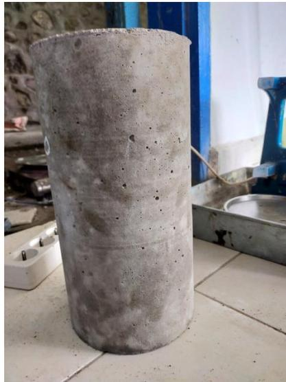
**Gambar 3. 1** Benda uji selinder 300 mm × 150 mm
