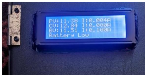
**Gambar 4. 8** Pengujian under voltage
