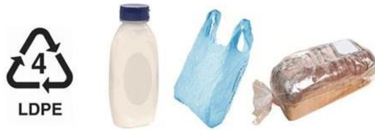
Gambar 2. 4 Plastik LDPE ( Low Density Polyethylene ) (Sumber: Google, 2024)
