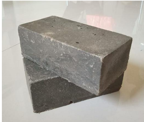
Gambar 3. 1 Benda uji paving block 21 cm x 10,5 cm x 8 cm
