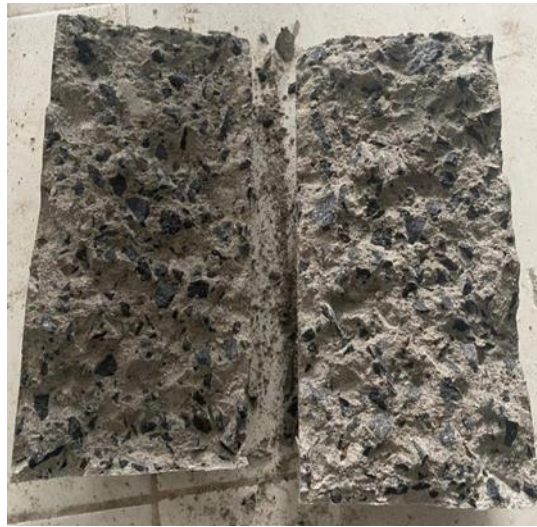
Gambar 9. Tarik Belah Beton Serat Fiberglass 1%
