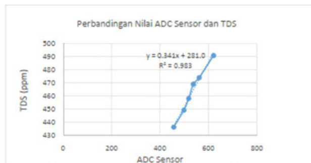
Grafik 8. Karakteristik nilai ADC sensor terhadap nilai TDS sensor kalibrator TDS meter (uji TDS)
