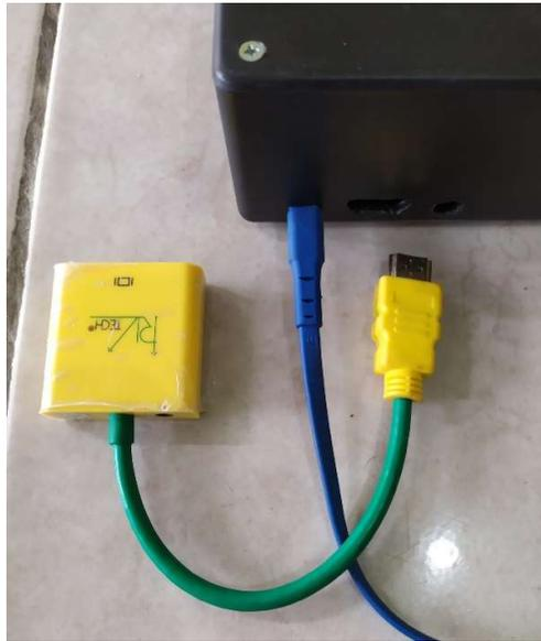
**Gambar 4. 30.** *Hdmi to vga converter*
