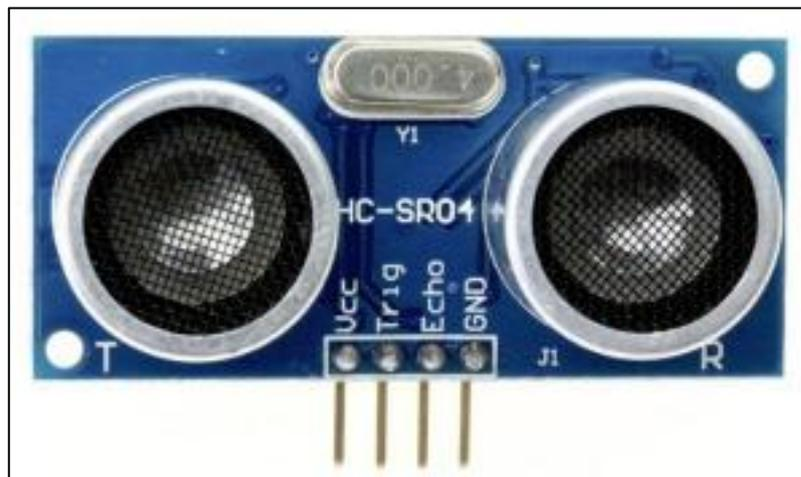
Gambar 2.2 Sensor Ultrasonik
