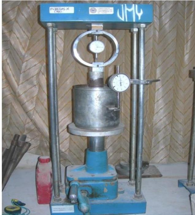
**Gambar 2.4** Alat California Bearing Ratio (CBR)
