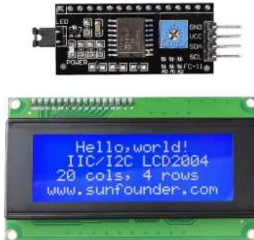
**Gambar 2.9** LCD 20x4 I2C
