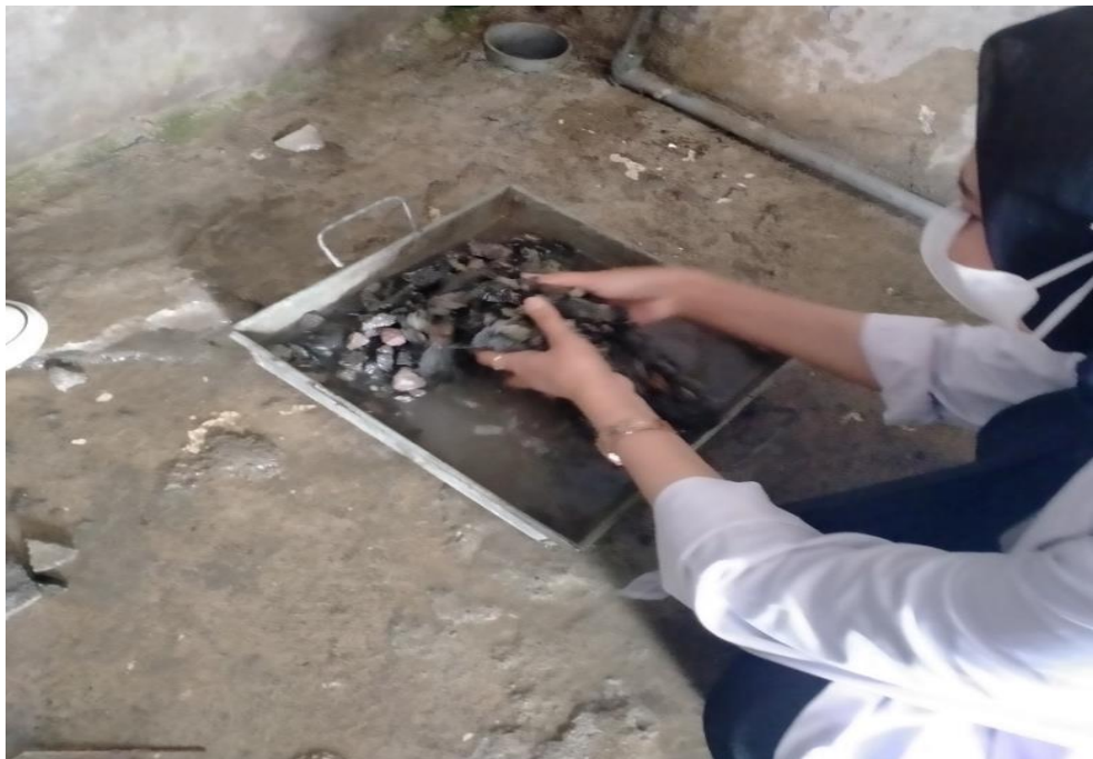
Proses Pencucian Agregat
