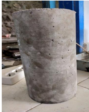
Gamar 3. 14 Benda uji silinder 300 mm × 150 mm
