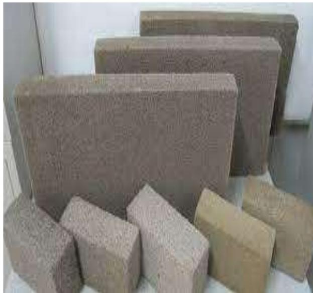
**Gambar.2.7.** Air Entrained Concrete atau Foam Concrete
