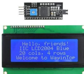
Gambar. 2 4 *Liquid Crystal Display 20x4*
