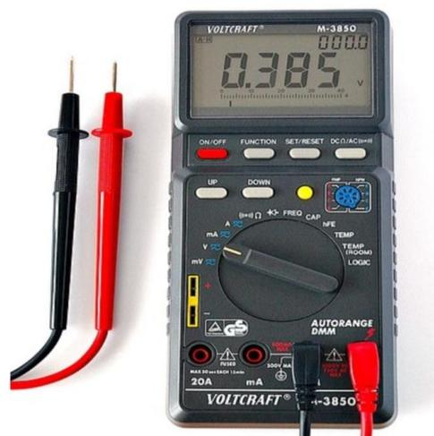
Gambar 4.12 Multimeter
