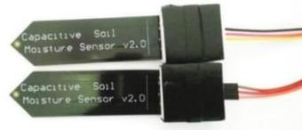
Gambar. 2.3 Sensor *Soil Moisture*
