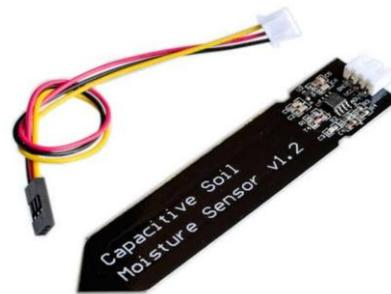
Gambar 4.9 Sensor *Soil Moisture*
