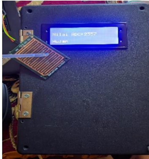
Gambar 7. Proses pengujian sensor raindrop
