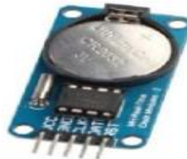
Gambar 2.5 Real time clock ( sumber : Suryadi, 2017)
