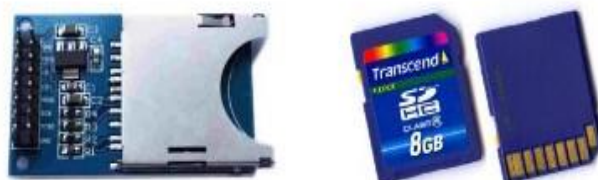
Gambar 2.6 Modul SD Card ( sumber : Pratama,2021)
