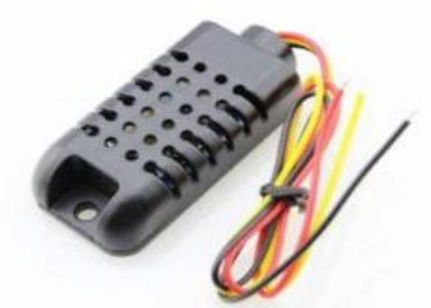
Gambar 2.2 DHT21 ( sumber : Kurniawan, dkk, 2023 )
