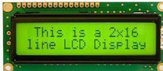
**Gambar 2.6** LCD (Liquid Crystal Display)
