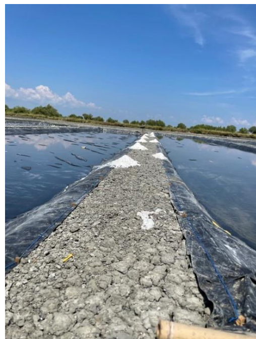
Figure 3. Salt production using geomembrane technology in Bulu Cindea village, Bungoro Sub-district, Pangkep Regency
