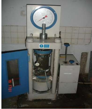
Gambar. 19. Combined UTM and ME frame
