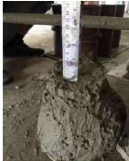
Figure 7.1. Slump Test.
