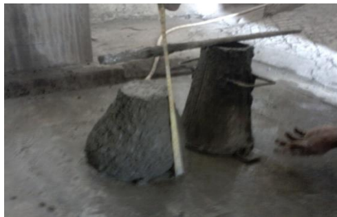
Gambar 5.1 Slump test beton normal
