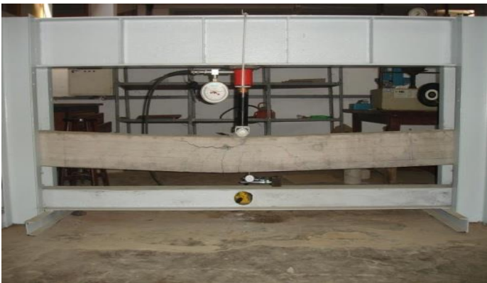
Gambar 5.10 Pola runtuh beton self compacting concrete
