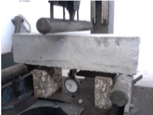
Gambar 5.4 Pengujian Kuat lentur Beton Self Compacting Concrete
