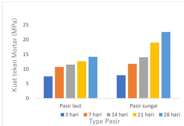
**Figure 3.** Comparison chart of compressive strength of sea sand and river sand mortar
