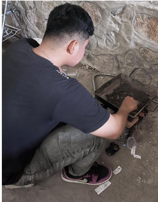
Pengujian kadar lumpur agregat halus pasir
