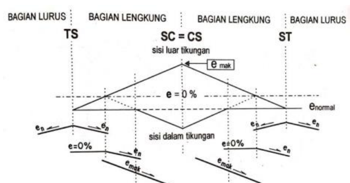
Gambar 2. 14 Diagram Superelevasi Spiral-Circle-Spiral Sumber : Pedoman Desain Geometrik Jalan 2021
