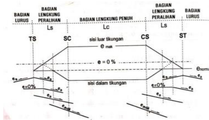
Gambar 2. 14 Diagram Superelevasi Spiral-Circle-Spiral Sumber : Pedoman Desain Geometrik Jalan 2021
