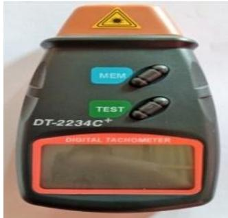
**Gambar 2. 2** Tachometer DT-2234C<sup>+</sup>
